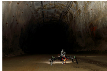
Inspection of tunnels with quadrotors
